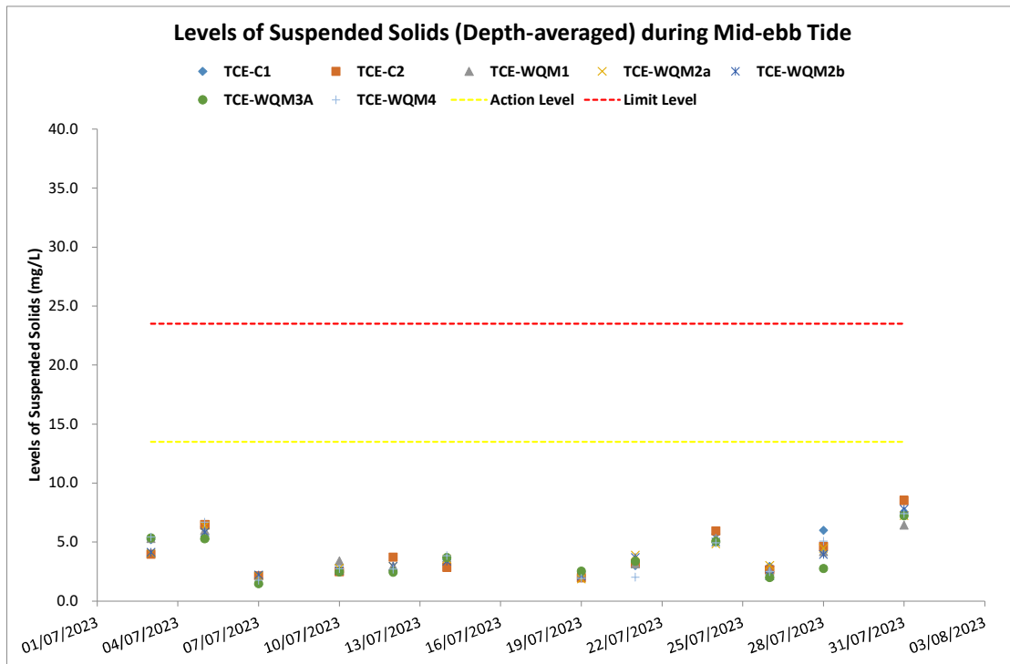
Figure 7: Levels of Suspended Solids (Depth-averaged) (mg/L) recorded at Mid-ebb Tide during the Water Quality Monitoring between 1 to 31 July 2023
